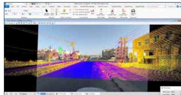
Figure 8. TopoDOT software point cloud overlaid over images
