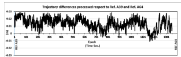
Figure 6. Differences in the Height of trajectory processed using different Reference Stations with a 10km-distance from each other
